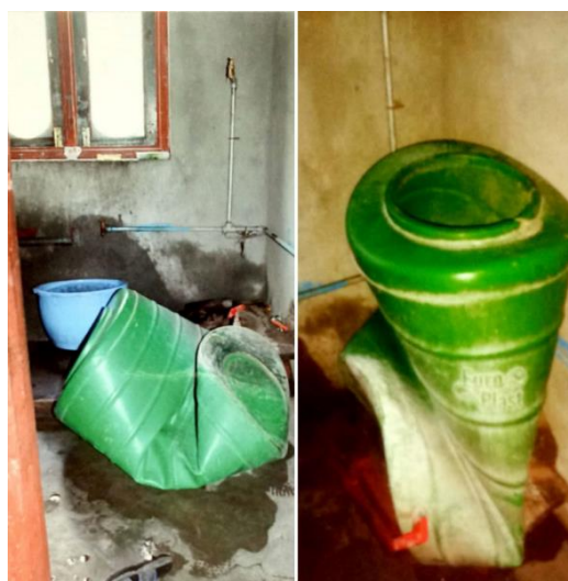
Fig. 2: Overheated Molten Deformed Plastic Water Tank
